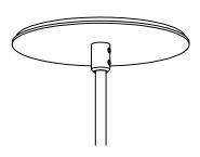
Mounting Option Power 2-5 65mm Diameter Box (By Others) Installed in drywall, wood or concrete ceiling
